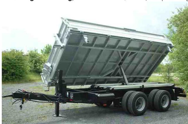
**Total weight 18000 kg**, order number 889/18000, net load approx. 13800 kg, loading gauge approx. 5000x2420 mm, loading height unloaded approx. 1110 mm, twin tired (eight tires) accessories: feather jack and central locking
