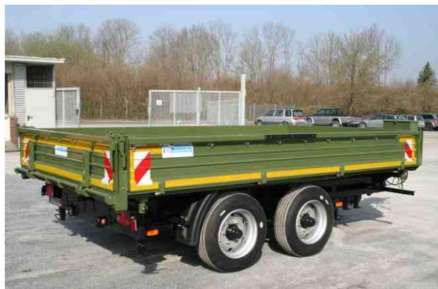
**Total weight 6900 kg**, order number 852/6900, net load approx. 4650 kg, loading gauge approx. 4000x2300 mm, loading height unloaded approx. 880 mm, accessories: tool box, warning stripe, hooks
